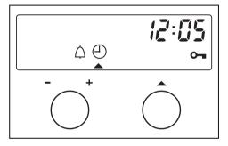
■ Turn the function selector (right hand dial) until triangle ▲ is underneath the ④ symbol in the display.
